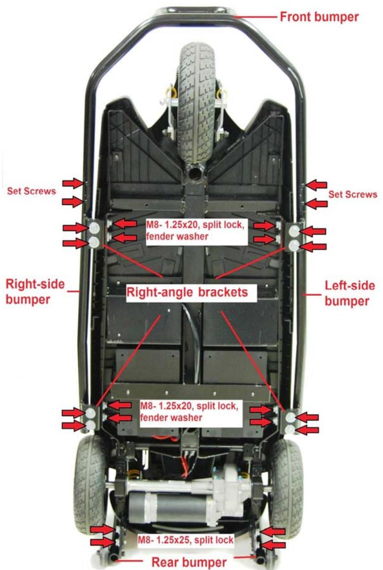
**Figure 3: Underside of Frame**
